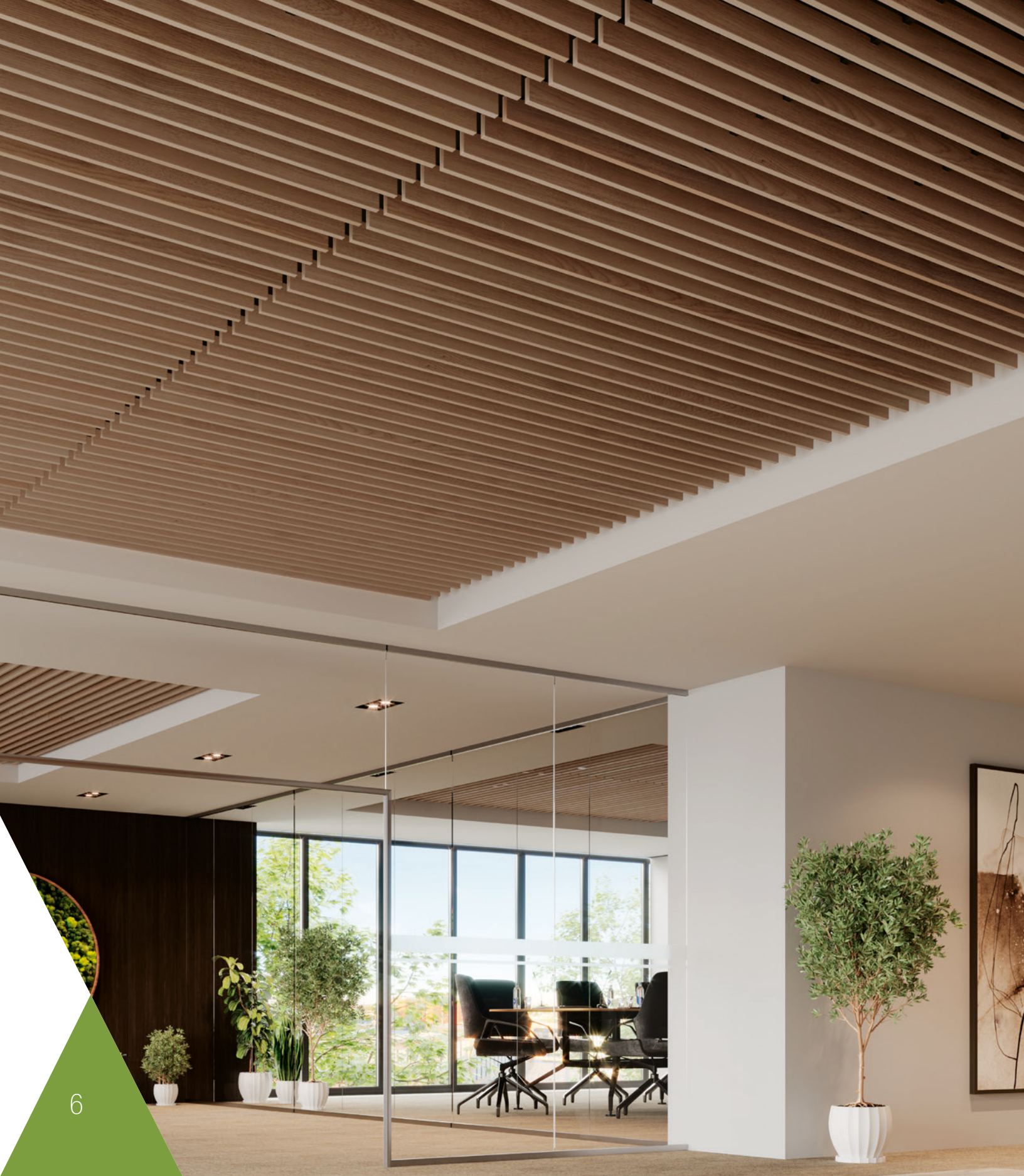
▲ WoodWorks® Grille – Forté veneered 3-slat panels, 3/4" W x 2-1/2" H in 96" lengths in Plain Slice White Oak (NOK)
