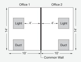
2. Poor design – 2' x 2' lights 2 ft. from common wall, 2' x 2' open grill return 2 ft. from common wall (no boot).
