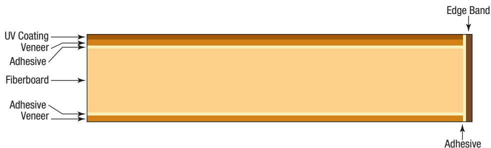
Figure 1. Composition of a WoodWorks® ACGI Ceiling Panel
