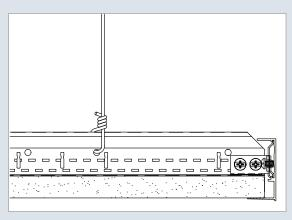
Section cut detail provided in the ProjectWorks Drawing Package, illustrating how the system is installed.
