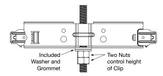
In cases where additional bracing is required, it may be acceptable to support the CLP7301 Clip using hanger wires
