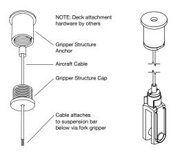
**Note:** In cases where attachment to structure is not possible at 24" centers, hanging kit assemblies can be spaced at a maximum of 36" OC along the length of the bar and within 12" of each end of the bar. (holes for the Attachment Pin will have to be drilled in the field).
