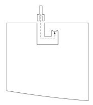
Each blade is attached to the suspension system by means of hanging the factory hook cut out in the blade over the vertical flange of the suspension bar.
