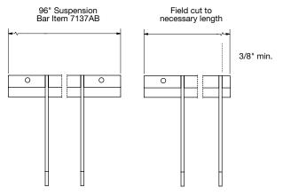
To touch up cut ends of the suspension bar, use a commercially available matte black paint.
