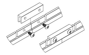
9. At the perimeters of the installation the suspension bars can be cut to length (see below). The suspension bars are extruded aluminum and it is recommended that they are cut with a metal cutting chop saw or battery powered circular saw. When cutting to length, be sure to leave at least 3/8" of material from the last notch to the end of the suspension bar.
