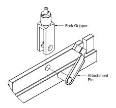
Slip the attachment pin through the fork and hole in the suspension system and secure the attachment pin to the top of the fork gripper.
