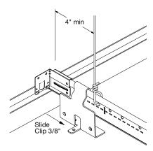
**NOTE**: When BERC2 is used, the clips adjacent to the molding must be relocated 3/8" toward the center of the panel. Draw lines through the factory-drilled pilot holes across the back of the panel. Shift the outer clips 3/8" toward the center of the panel and secure each with three screws.
