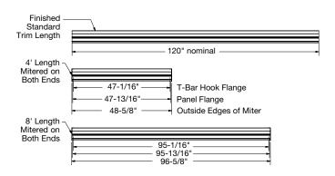
Test one piece of trim running the length of install to make sure the FXTBC clips are positioned correctly (measurement from T-Bar hook flange to cross tee should be 23-1/16" – standard 24" x 24" suspension system opening).
