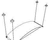
FOR EACH HANGING KIT THAT IS SPECIFIED, INCLUDE ONE ESCUTCHEON KIT TO PROVIDE A COVER FOR THE HOLE CREATED IN THE EXISTING CEILING.
