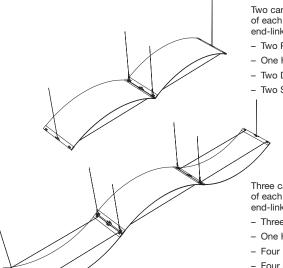
Two canopies linked and suspended with one cable at one end of each canopy, and two new dual canopy cables between end-linked canopies, you need:
