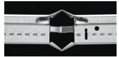
Main beam exposed to fire
