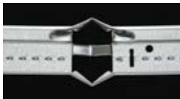
Main beam exposed to fire
