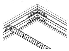
To secure splice plates for straight trim joints, pull the trim tightly together for the best fit. Use a 1/8" hex key wrench to tighten the set screws that secure splice to trim. CAUTION: Do not over-tighten these screws to the point where they distort the face of the trim.
