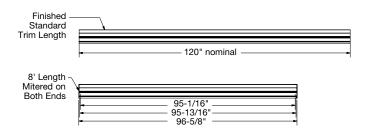
Test one piece of trim running the length of install to make sure the FXTBC clips are positioned correctly (measurement from T-Bar hook flange to cross tee should be 23-1/16" – standard 2' x 2' grid opening).
